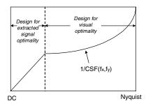
Figure 2. The carrier is designed for extracted signal quality for low spatial frequencies and visual optimality for high spatial frequencies
